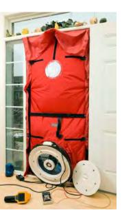
House undergoing a blower door test. Test provides a measured air leakage rate and can help identify areas in the building envelope that need to be addressed to improve airtightness.
